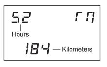
of kilometres that the walking belt has moved. An "M" for metric kilometres or an "E" for English miles will appear in the Pace/Speed zone. Press the Speed increase button to change the unit of measurement if desired.
